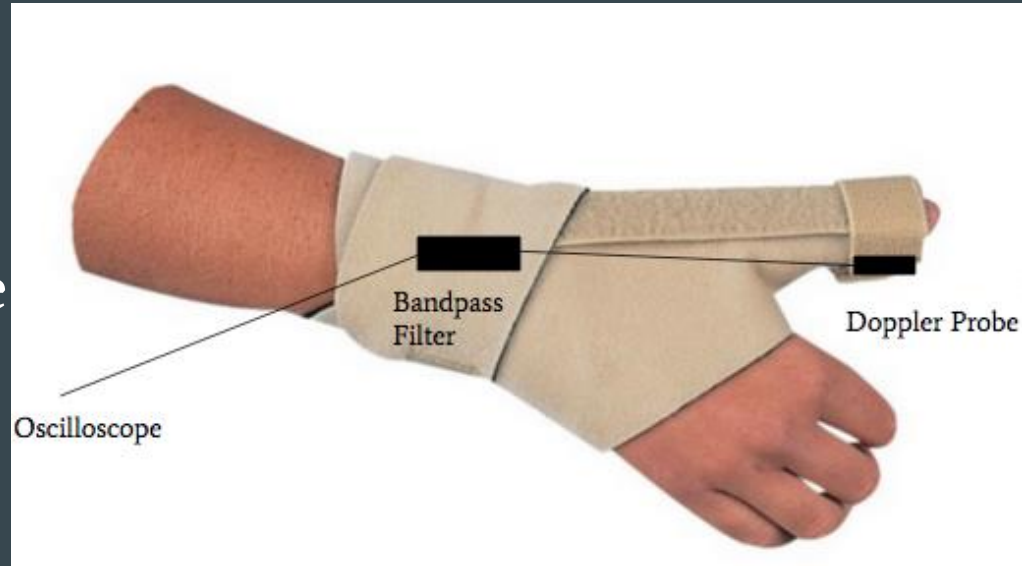
Figure 6- Splint design with added bandpass filter [5]
