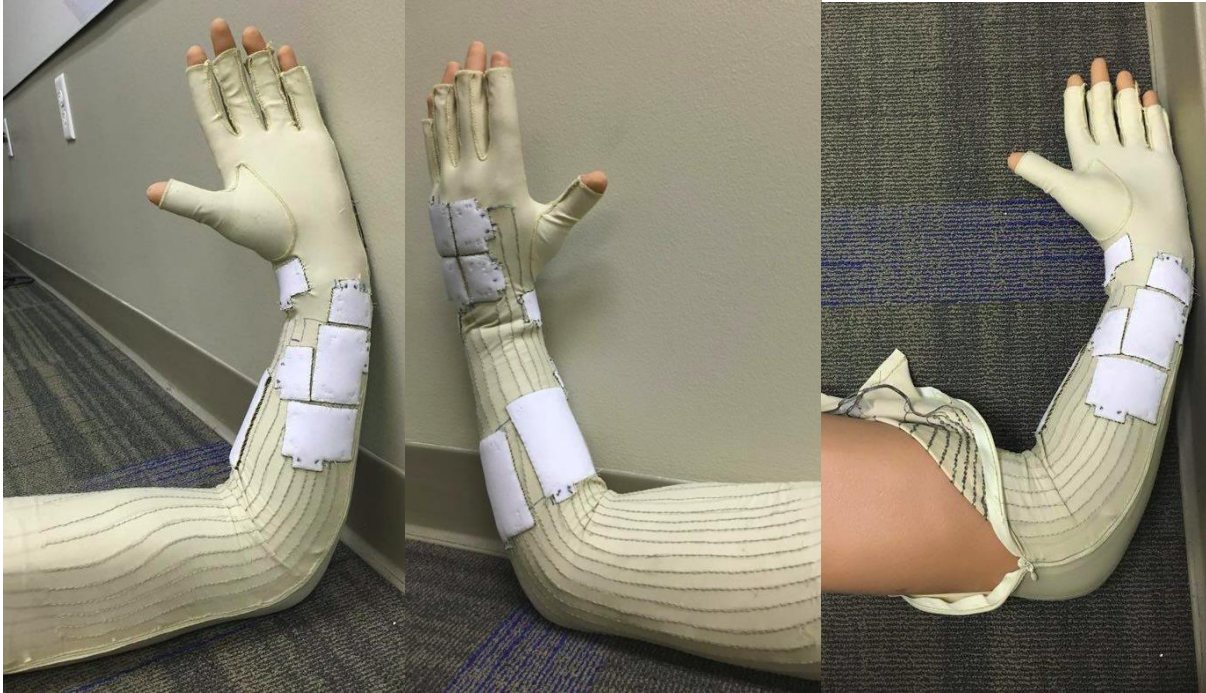
Figures 14, 15, and 16: These images show the final product at multiple angles in order to display all of the sensors and the interior conductive thread.
