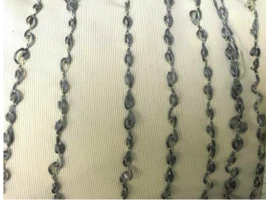
Figure 8. Knit stitch off conductive thread on underside of edema glove
