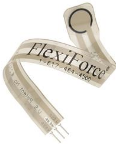
Figure 1. FlexiForce Sensor. This image displays the small round sensing area of the FlexiForce Sensor with the attached flexible leads [4].
