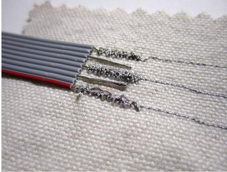
Figure 3. Conductive thread sewn into material and connected to wires using a zigzag stitch [10].
