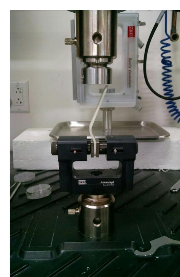
Figure 9: MTS setup of ABSplus plastic prototype
