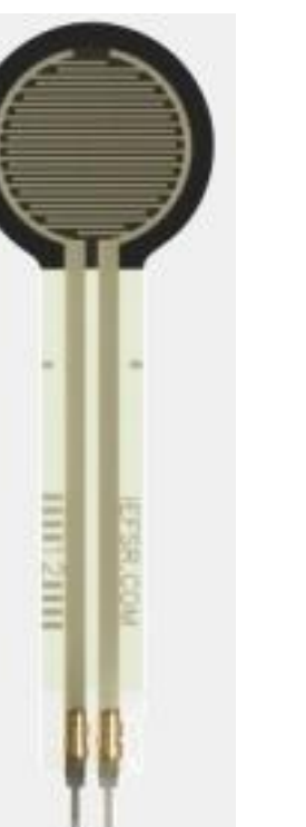
Figure 13: Intertek 402 FSR used to determine the forces exerted on the leg by the hinge
