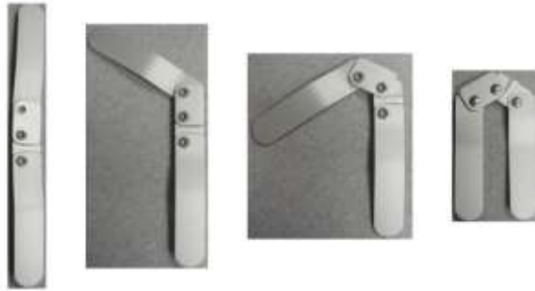
Figure 4: The Tri-Axial Hinge, made of four parts connected by bolts and capable of 180° of motion.
