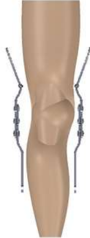
Figure 9: Image on how the Adjustable-Hinge design would conform to each side of knee.
