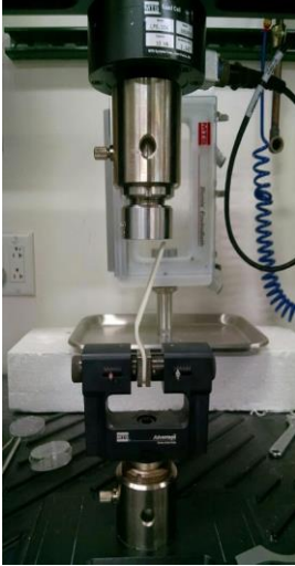
Figure 20: MTS Testing. To perform the MTS testing, the Y-arm was gripped on the bottom of the 3-D printed part that connects to the rest of the hinge. A flat load cell was used to compress the piece due to the angled shape of the design.
