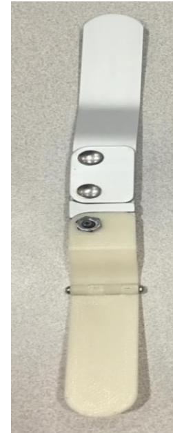
Figure 19: Adjustable-Hinge. The distal end that was 3D printed was attached to the current hinge and two screws were inserted in opposite directions.
