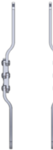
Figure 5: Side view of Tri-Axial Hinge. The Tri-Axial has a straight leg profile, causing pressure in the upper thigh.
