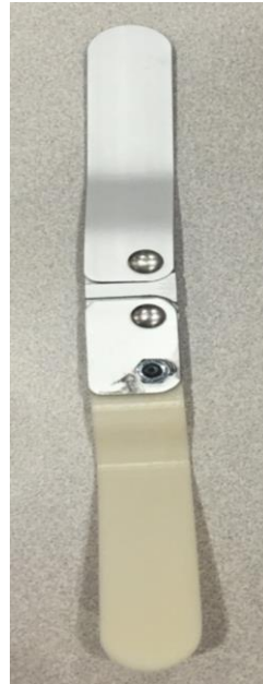
Figure 18: Y-arm. The distal end that was 3D printed was attached to the current hinge.
