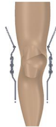
Figure 13: The Adjustable-Hinge in Relation to the Knee. The Adjustable-Hinge allows the user to set the angle of the distal end to conform to their thigh size.
