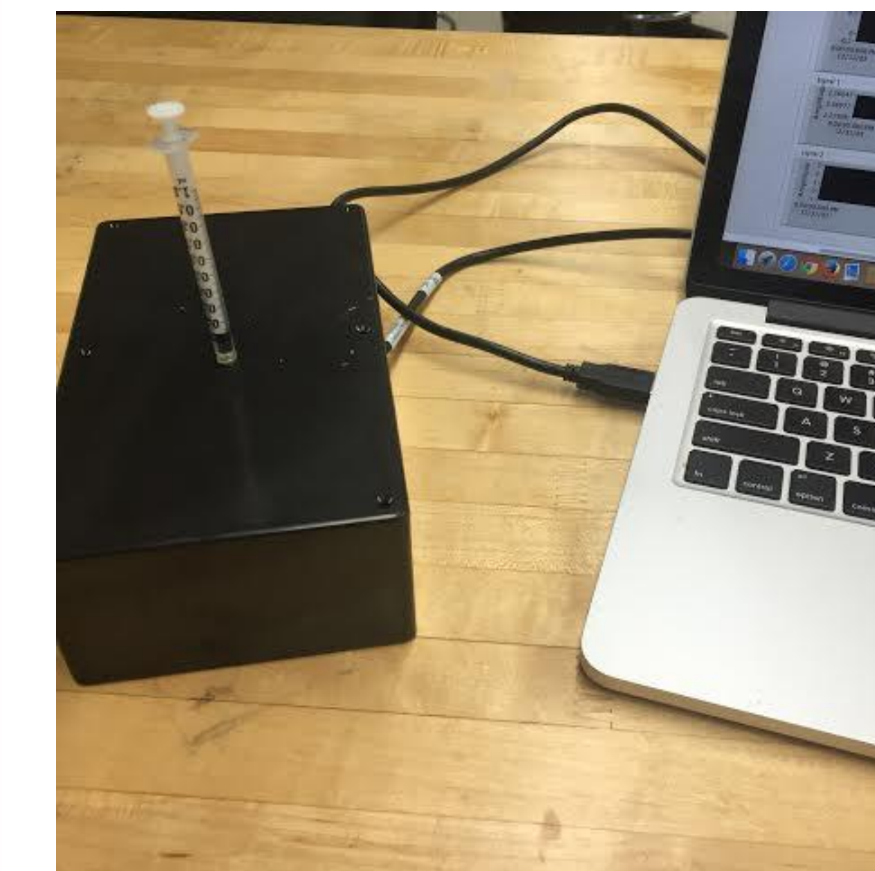
Figure 10: The box connects from the NI-DAQ to a computer which reads data through a custom LabView script
