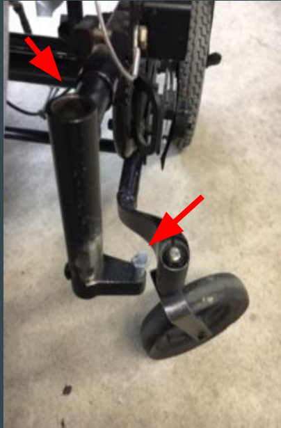
Wheelchair connection and locking mechanism pin
