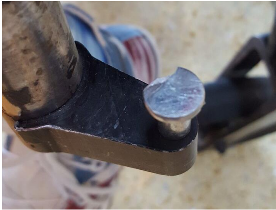
Figure 4. Breaking of Locking Mechanism Pin
