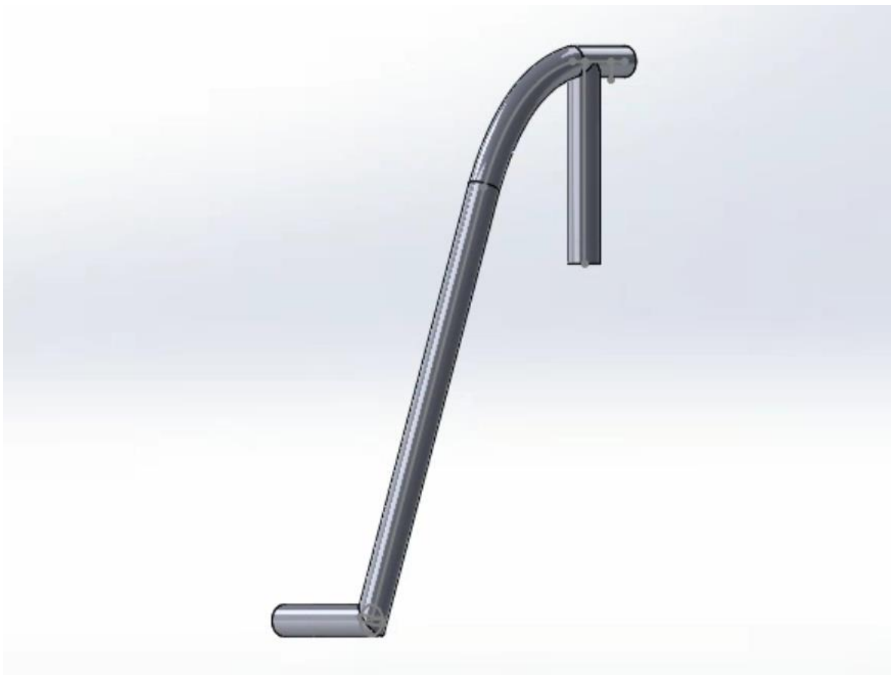
Image 3: SolidWorks Model of footrest rod only.
