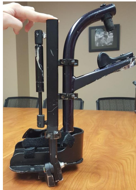
Figure 2,3. Current Footrests. The design features a two-pronged hanger which attached to the wheelchair frame via a point of rotation above and a bi-directional locking mechanism below. The hanger is attached to an extension bar, gas-loaded springs, and an angle adjustable footplate.
