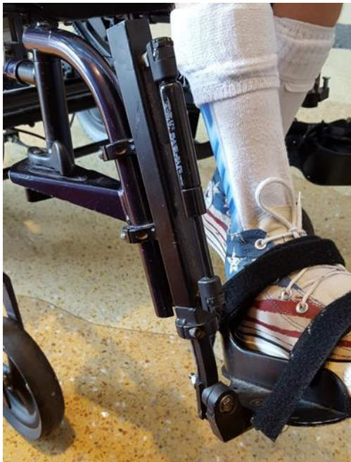
Figure 2,3. Current Footrests. The design features a two-pronged hanger which attached to the wheelchair frame via a point of rotation above and a bi-directional locking mechanism below. The hanger is attached to an extension bar, gas-loaded springs, and an angle adjustable footplate.
