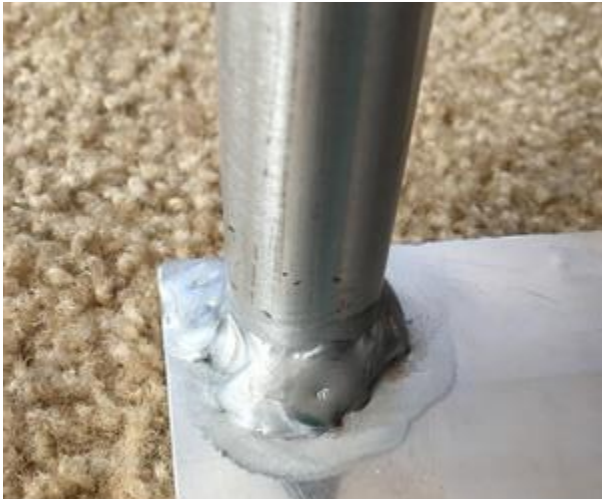
Figure 20. Weld between footplate and bar
