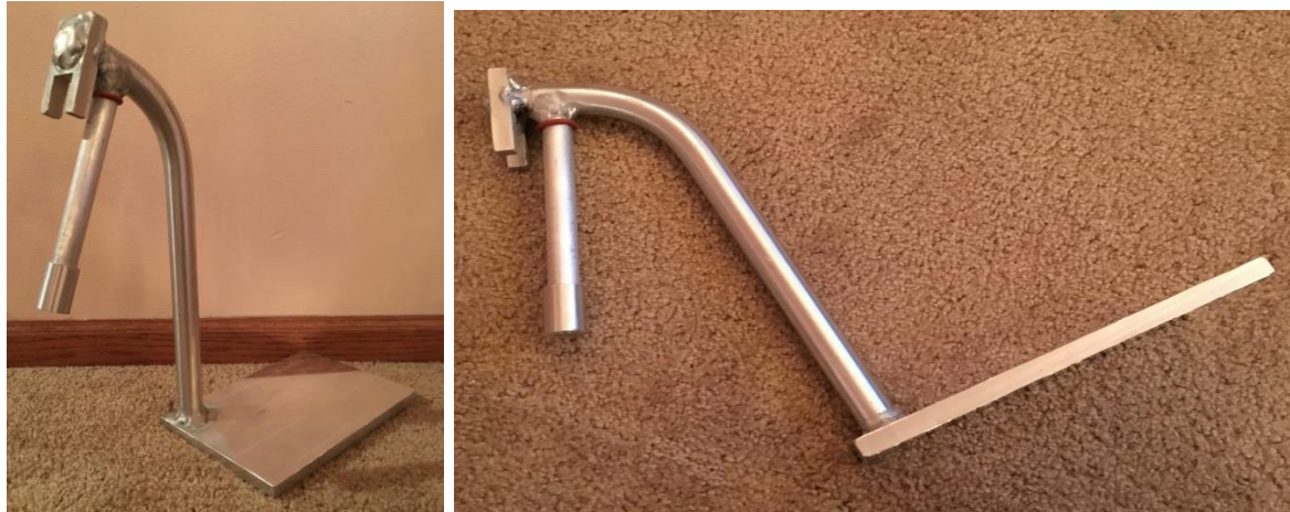
Figures 22, 23. Final Footrest Prototype.
