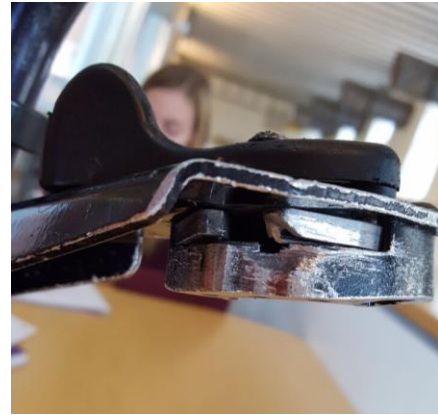
Figure 5. Wear of Locking Mechanism
