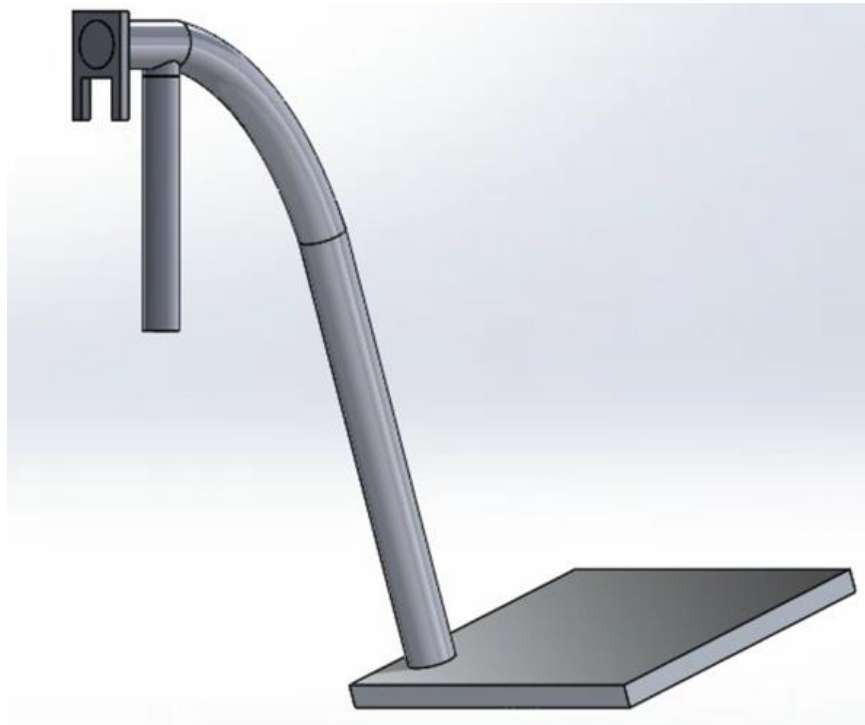
Figure 21. Final Prototype. The final extended hanger design features a hanger bar which extends further past the bent segment than the current footrests, a “U-Saddle” piece which prevents rotational motion by dropping down over the wheelchair frame bar, and a drop-down bar and cap which prevent
