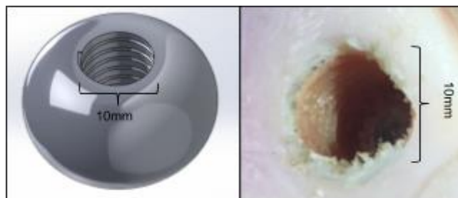
Figure 9: On the left is a SolidWorks model of the threaded recipient site, and on the right is the threaded recipient site in the femoral condyle of the cow femur
