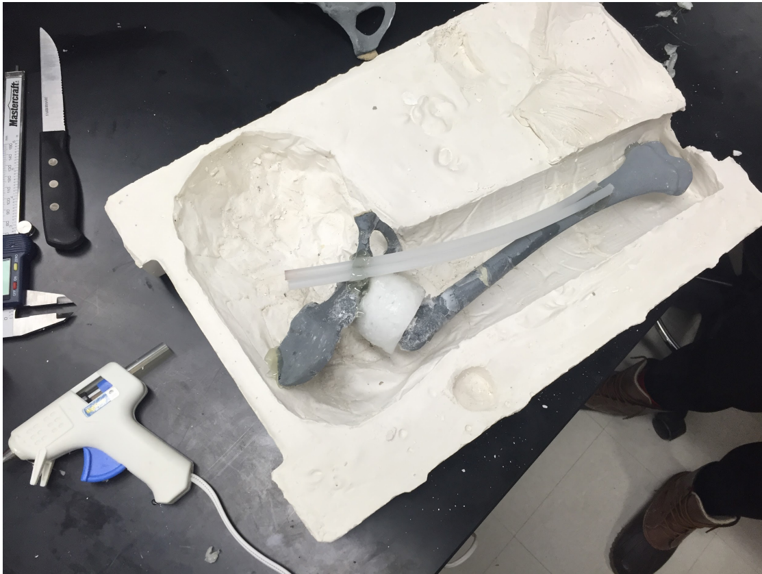
Figure 7: Placements of Bones within Plaster Negative
