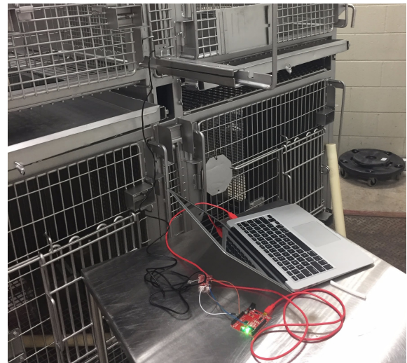
Figure 10: This image displays the testing setup of the device. The load cell's black wire is pictured running from the device to the Arduino circuitry on the desk. The circuitry is then connected to the computer, which is running the testing program.
