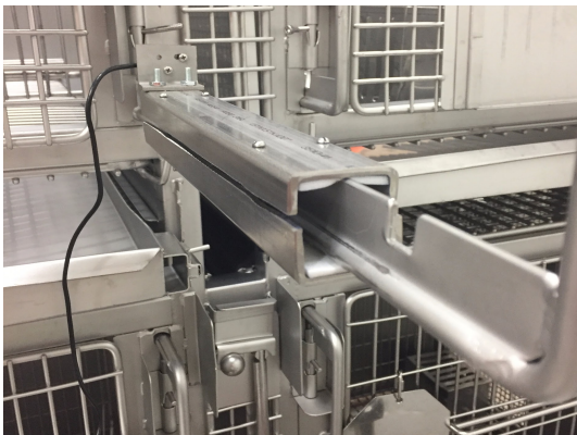
Figure 7: Above is an image of the final prototype facing the cage. The polyethylene foam can be seen forming to the squeeze plate bar, increasing frictional forces and keeping the device in place.
