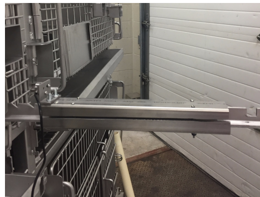
Figure 8: Shown is a side image of the attached final prototype. In this image the clamping mechanism can be seen. The four screws on the surface protrude out the bottom of the device and are held in place by firmly tightened bolts. On the cage side of this image the load cell can be seen attached to the device.
