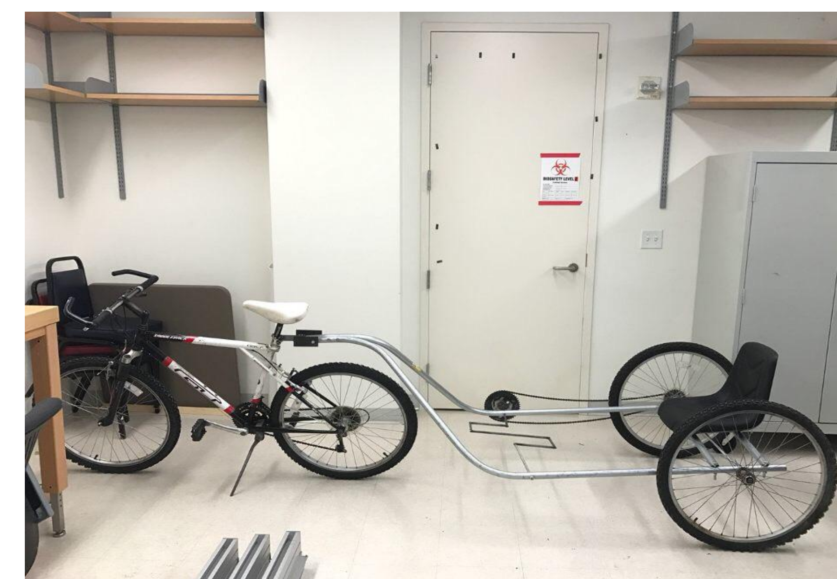
Figure 2: The finished prototype connected to the client's bike
