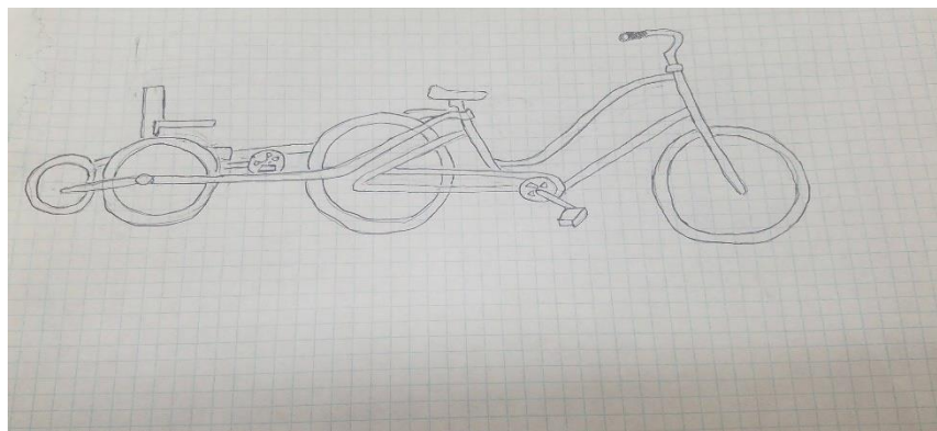
Figure 1: The trailer sidecar is attached to the seat of the driver's bicycle.
