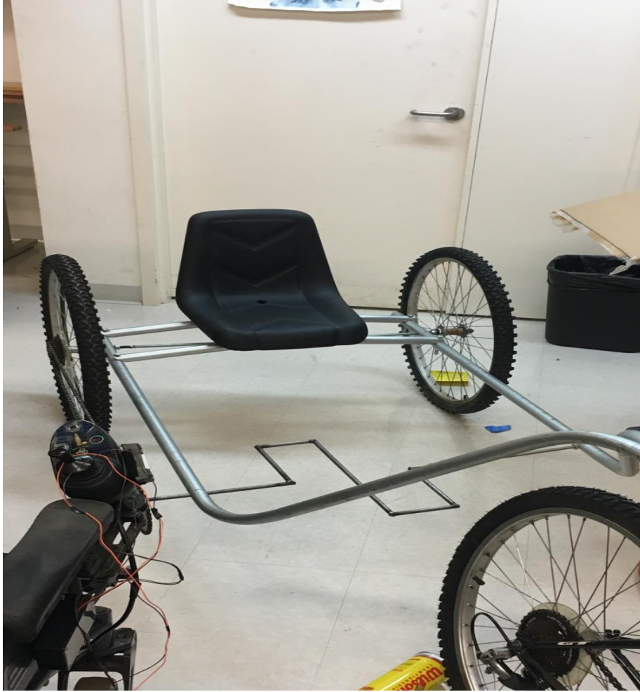
Figure 6: A final prototype consisting of self-fabricated pedals, a gear system similar to a paddle boat, and a padded seat on a positively bent bar.
