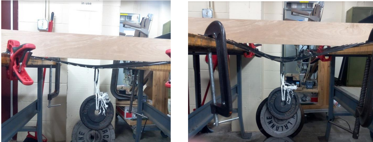
Figure 7. Top: A picture of mesh deflection testing setup with no initial weight. The wooden plank was used across the top of the mesh to reference a horizontal measuring point. Bottom Left: A picture of the 1" x 1" mesh with 50 lbs applied. Bottom Right: A picture of the 2" x 2" mesh with 50 lbs applied.
