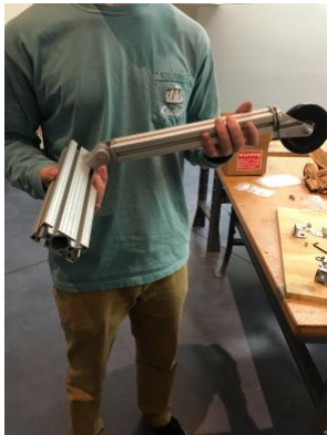
Figure 11: One of the rear legs attached to the back portion of the chair frame.
