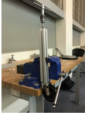
Figure 10: Tapping of the upper portion of the legs to allow for the attachment of the hinge. Hole for wheel has already been expanded and tapped, with wheel attached in image.
