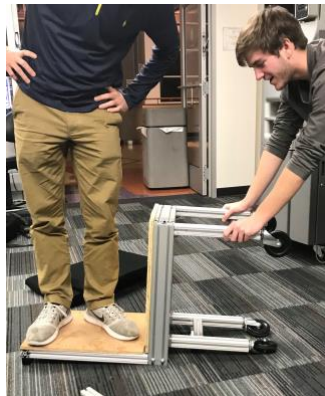
Figure 18 : Impulse loading test using weight of team member
