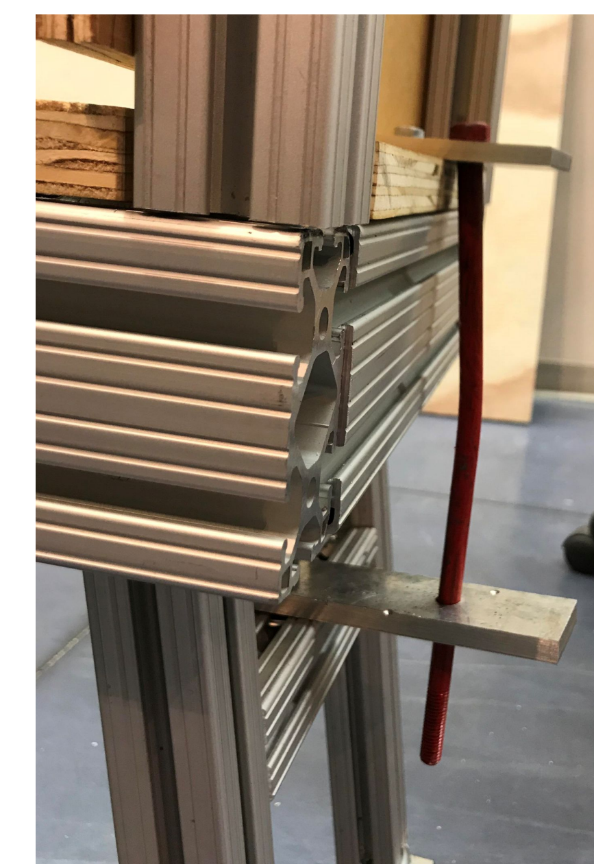
Figure 5: Initial failure of locking mechanism
