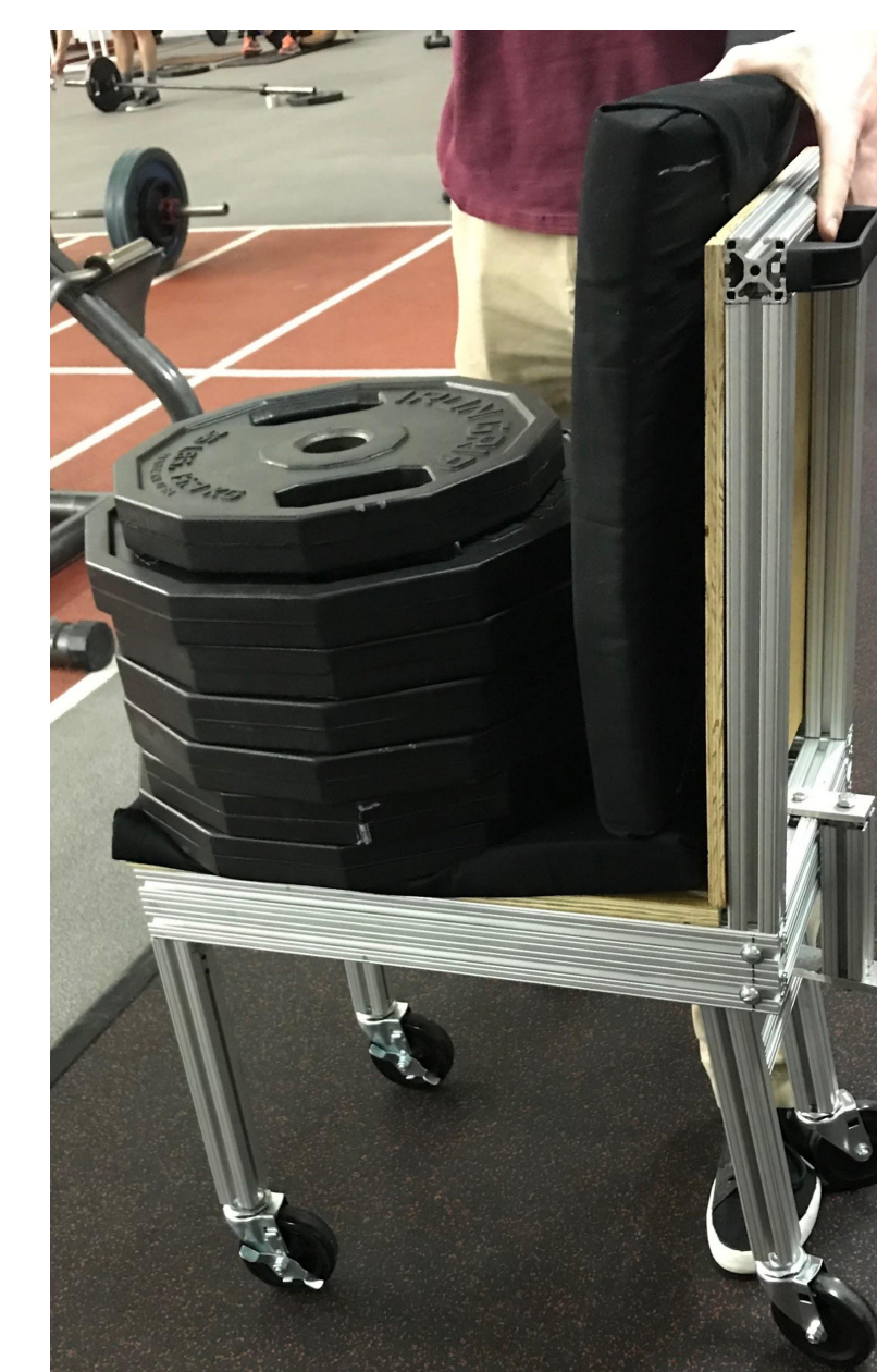
Figure 6: Static load test with chair holding 305 lbs
