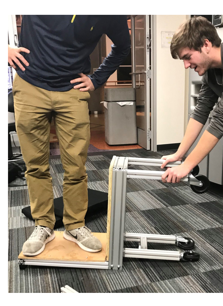
Figure 7: An impulse load is applied to simulate running into a bump.
