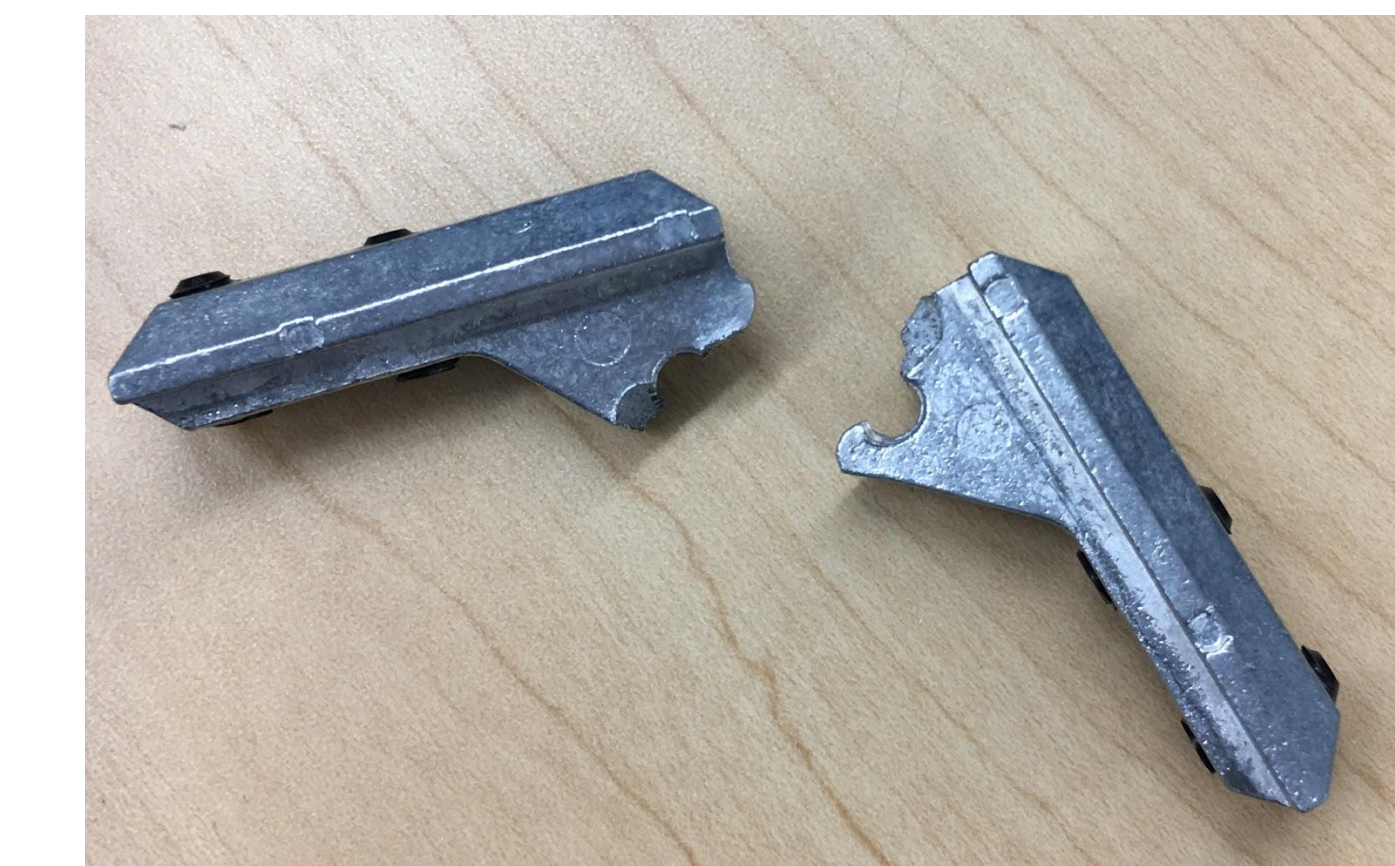
Figure 9: A failed joint resulted in a design change during testing
