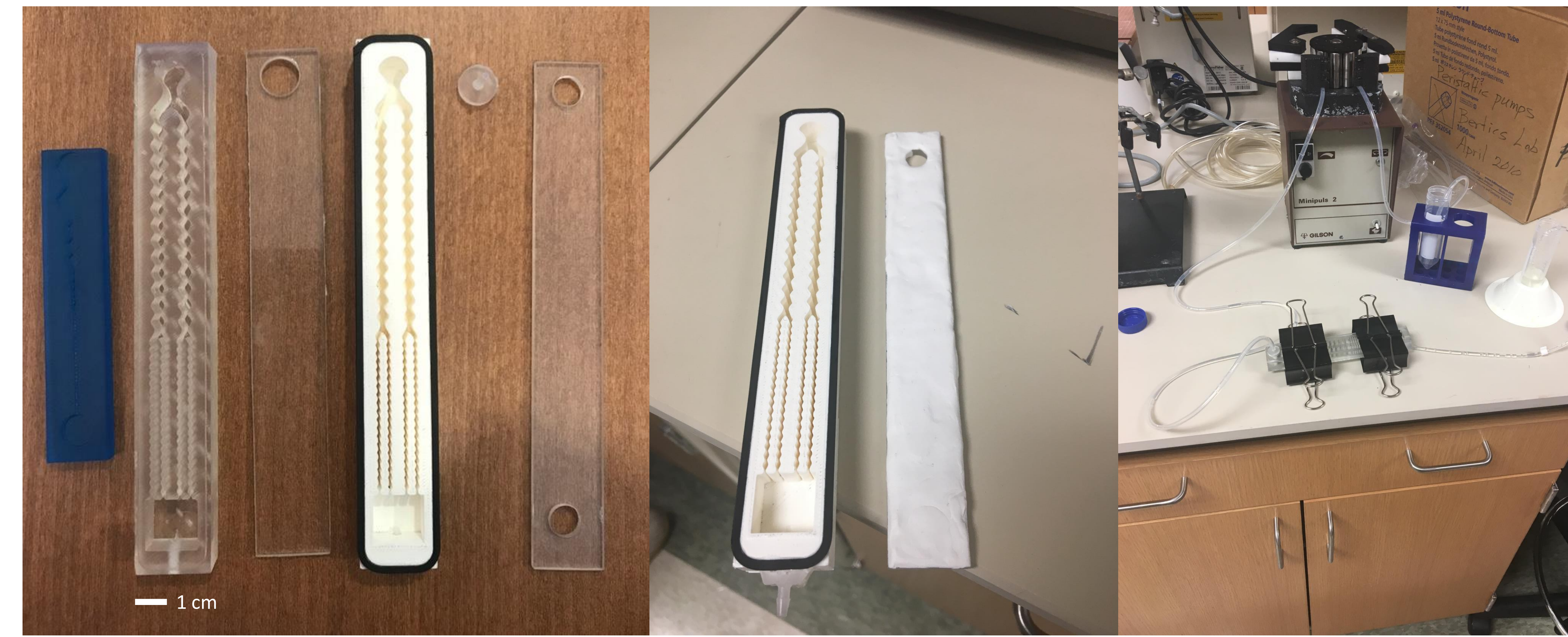
Figure 4: Design progress left to right. Left: Comparison of original design in blue to clear design and white design. The only difference between the clear and white design is that the white design has a rubber gasket around it to prevent leakage in the final design. Right: Final design in preliminary set up with makeshift clamps used for testing.
