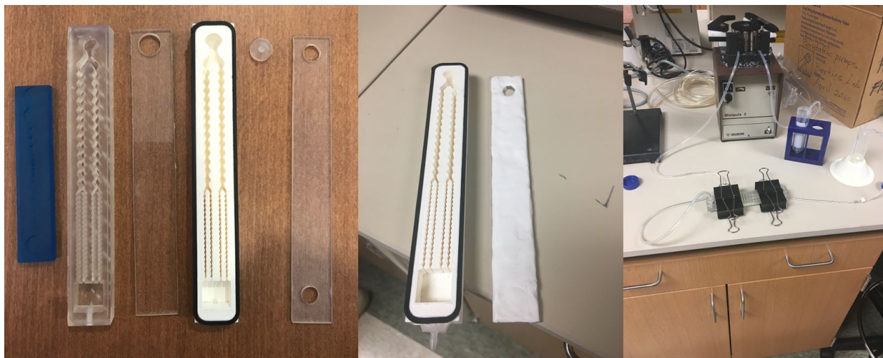
Figure 7: (Left) Initial device in blue compared with two final prototypes in clear and white. White was used for testing. Lids and adaptor are shown as well. (Middle) Final design with tubing adaptor and lid with rubber sealant used for testing. (Right) Testing set up with peristaltic pump, clamps for holding device shut, and tubing.
