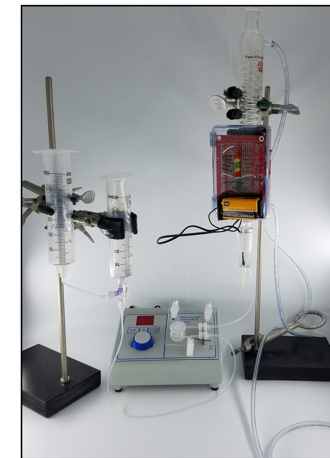
Figure 5. Final Langendorff Design
