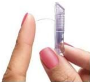
Figure 4: A Dexcom G5 glucose sensor shown to scale next to a human hand [12].
