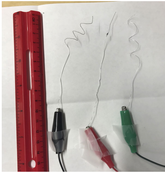
Figure 13: Three electrodes shown connected to the wires leading to the circuit. From left to right; reference, working, and counter electrode. The working electrode has been extended using silver Epoxy.
