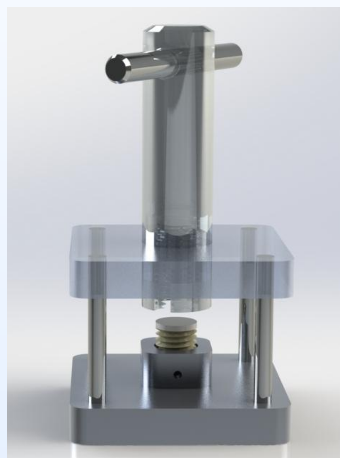
Figure 1: Solidworks Prototype Rendering. The bone plug is fixed in supporting cup. The guiding platform ensures axial alignment between the graft and die to produce consistent, accurate threads.
