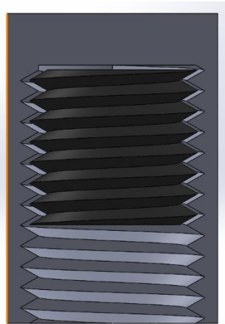
Figure 10: Retracted screw configuration of combined Tap and Die design.
