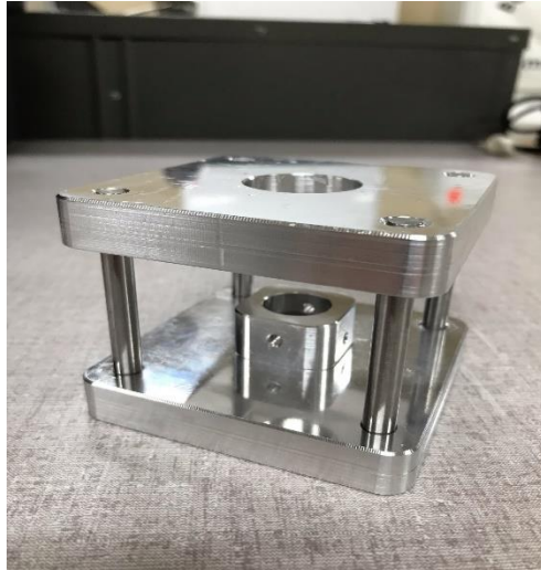
Figure 14: The die guiding platform was made from 6061 aluminum alloy for both flat faces, and stainless steel for all four dowel pins. The top face has a circular hole coinciding with geometry of the die for consistent threading of the graft. Here, the removable graft receiving cup, also 6061 aluminum, is placed into the square cut portion of the bottom aluminum face, preventing rotation while threading. Pin fixation of the bone graft through side holes in the graft cup also performs this function.
