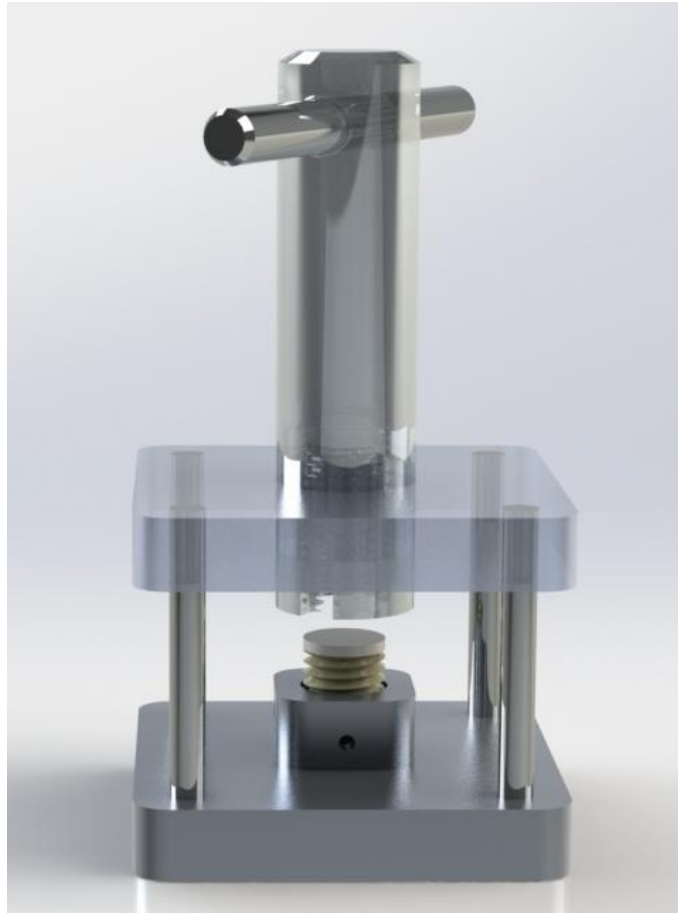
Figure 13: Solidworks rendering of the final die in the alignment plates with the threaded graft in the graft holding cup. This image demonstrates the intended interaction between these components to successfully thread the bond graft.
