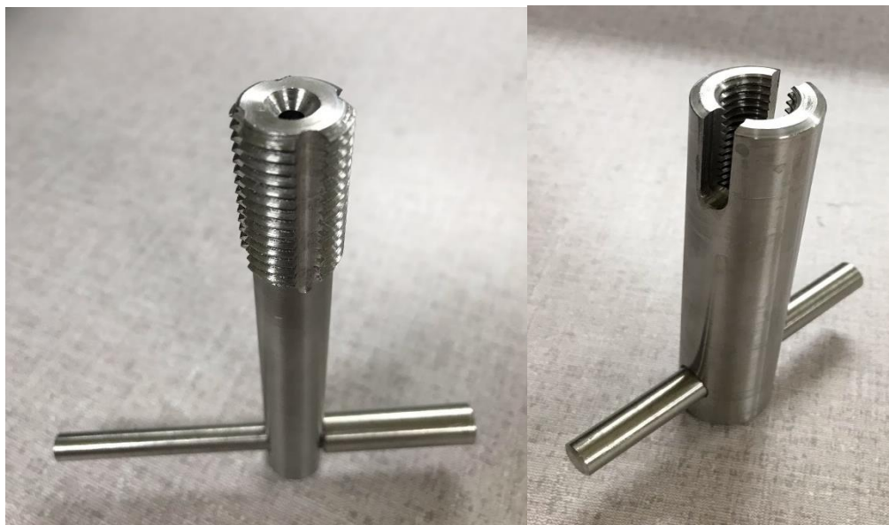
Figure 14: The die guiding platform was made from 6061 aluminum alloy for both flat faces, and stainless steel for all four dowel pins. The top face has a circular hole coinciding with geometry of the die for consistent threading of the graft. Here, the removable graft receiving cup, also 6061 aluminum, is placed into the square cut portion of the bottom aluminum face, preventing rotation while threading. Pin fixation of the bone graft through side holes in the graft cup also performs this function.
