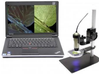
Figure 3. Dino-Lite Fluorescent Microscope [9]. A small handheld microscope that connects to your computer.
