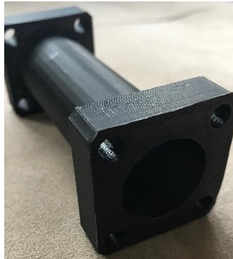
Figure 21. 3D-Printed light source tube. This tube connects the light source that is attached to the heat sink. The dimensions align to the size of the cage plate that contains the emission filter inside, which will all be attached to the side of the dichroic filter cube.
