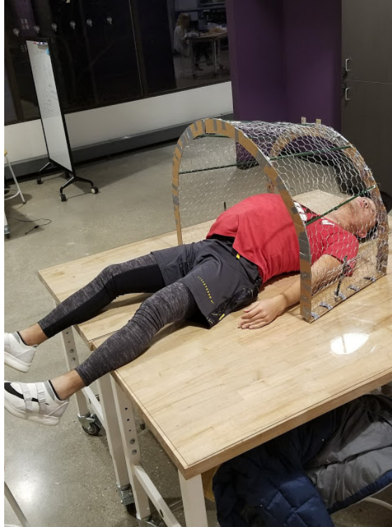
Figure 17: Depiction of how the shield is oriented with respect to the patient, the smaller arch is on the side nearest to the patient's head.
