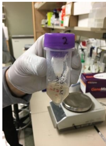
Figure 13: Hydrogels, tissue, and enzyme solution in gentleMACS conical tube during testing
