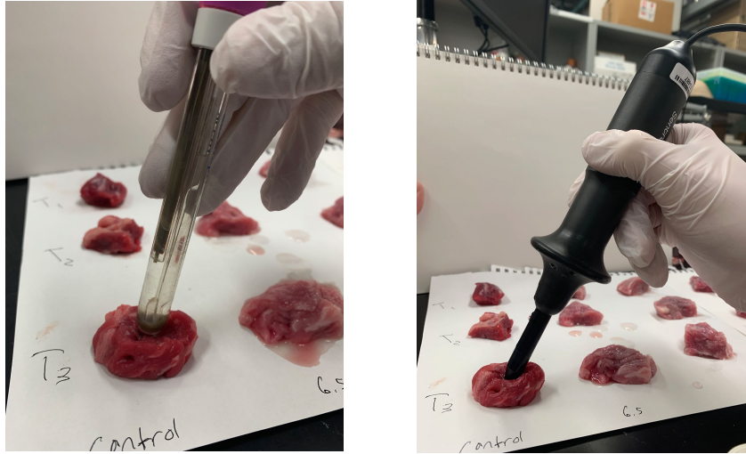
Fig. 10: Left: Insertion glass bulb pH probe into a buffer-soaked meat sample. Right: Insertion of the ISFET probe into a buffer-soaked meat sample.
