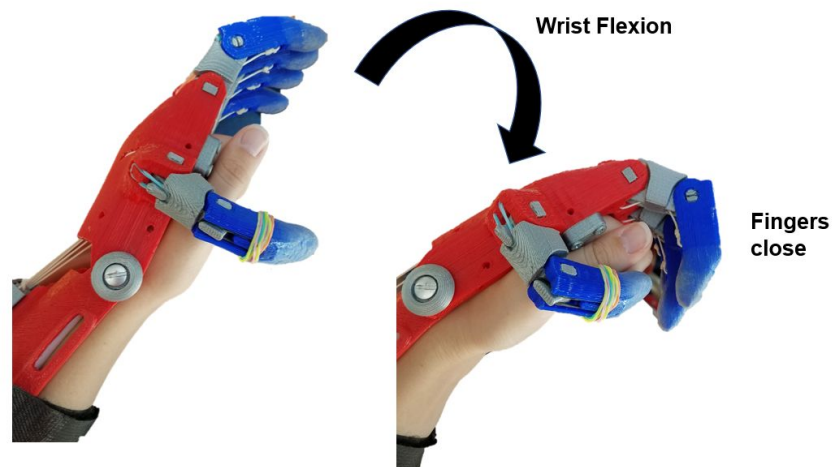
Figure 3: e-NABLE Hand Closure Mechanism
