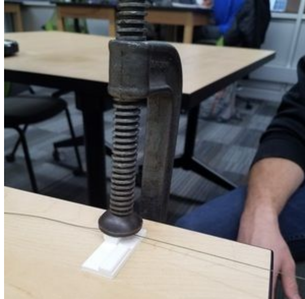
Figure 11: Testing setup. A corresponding upper piece made of either PLA or TPU was placed on either wavy or jagged side of the base for testing. String attached to a force gauge sits in between the upper and lower pieces, while the c-clamp was used to keep constant pressure on the two test pieces throughout testing.
