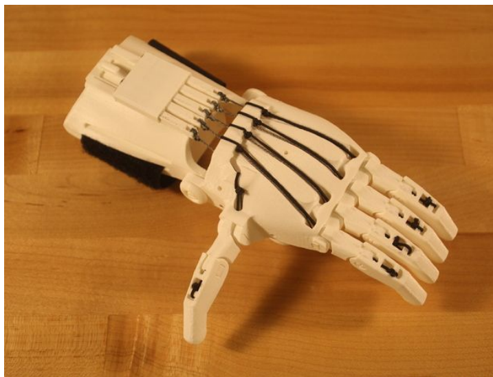
Figure 1. 3D printed and fully assembled Raptor Reloaded e-NABLE hand.
