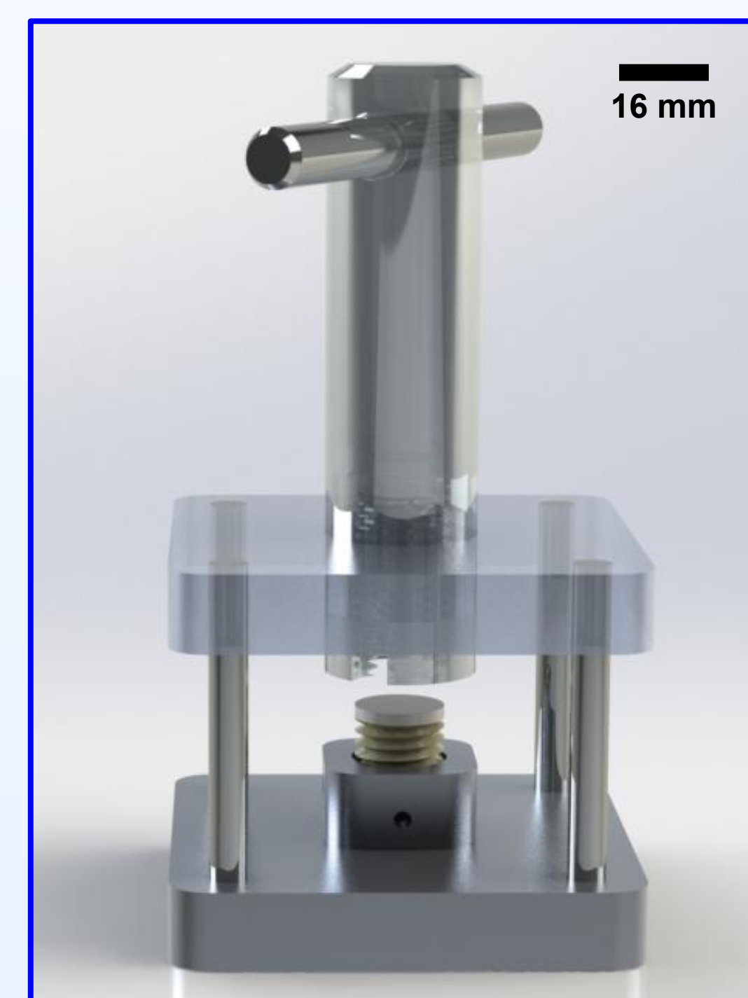
Figure 2: Solidworks Prototype Rendering. The bone graft is fixed in supporting cup. The guiding platform ensures axial alignment between the graft and die to produce consistent, accurate threads.
