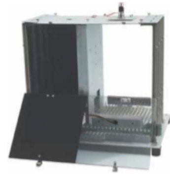
Fig 2. A rat passive avoidance cage by Coulbourn Instruments. Image taken from https://www.coulbourn.com
