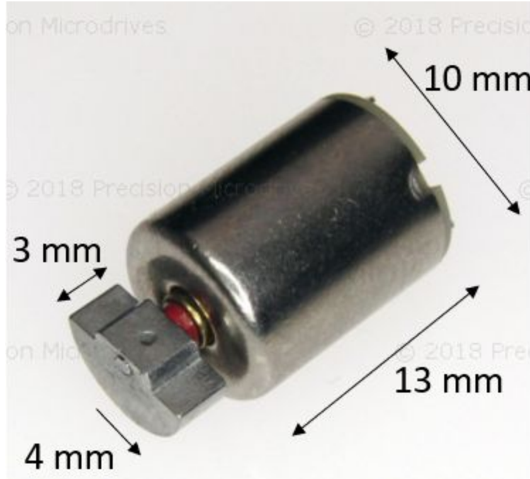
Figure 7. Precision Microdrives™ Model No. 310-112. The motor chosen for use in the proposed final design. The motor's adjustable frequency, as well as small size and low cost made it the preferred source of vibrational stimulation.
