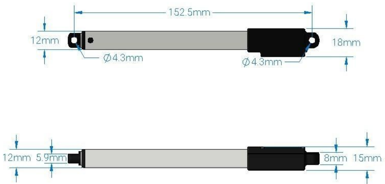
Figure 4. Linear actuator capable of one-dimensional linear movement [6]. The linear actuator allows for adjustable amplitude, and potentially adjustable frequency.
