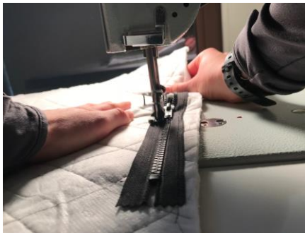
Figure 14: Team members sewing zippers to insulating fabric during fabrication
