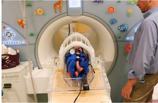
Figure 6: Visual depiction of the bore of an MRI scanner, as well as the head shield the infant warmer must accommodate [24]
