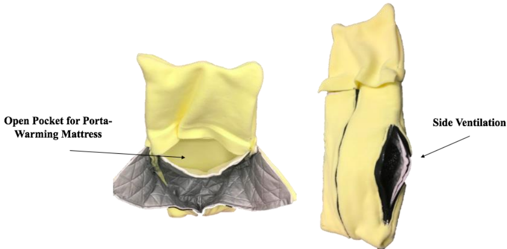
Figure 18: Visual representation of the “Sleeping Bag” with top-front view (left) displaying the pocket for the Cardinal Health Porta-Warming Mattress. The pocket is located between the fleece and insulating layers to hold a single Cardinal Health Porta-Warming Mattress which allows for active heat application to the baby without direct contact to the baby’s skin. The side-front view (right) displays the side vents for the removal of heat in case the infant becomes to warm. The vents can easily be activated in between scans and the zippers can be put at any desired position.
