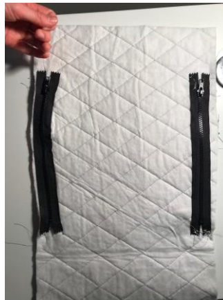
Figure 15: Photo of zippers sewn onto insulating layer showing progress during fabrication
