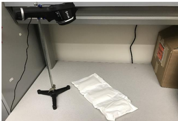
Figure 19: Testing set up with FLIR Thermal Camera fixed by a ring stand and heating pad below.
