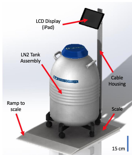
Figure 9: SolidWorks rendering of a standalone scale with an interactive LCD display.
