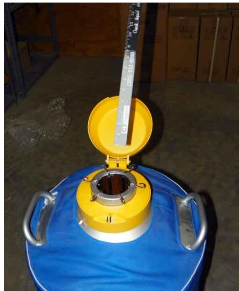
Figure 1. A measuring stick is a simple tool used to measure LN2 levels, colored black so that the frost line is easy to see.
