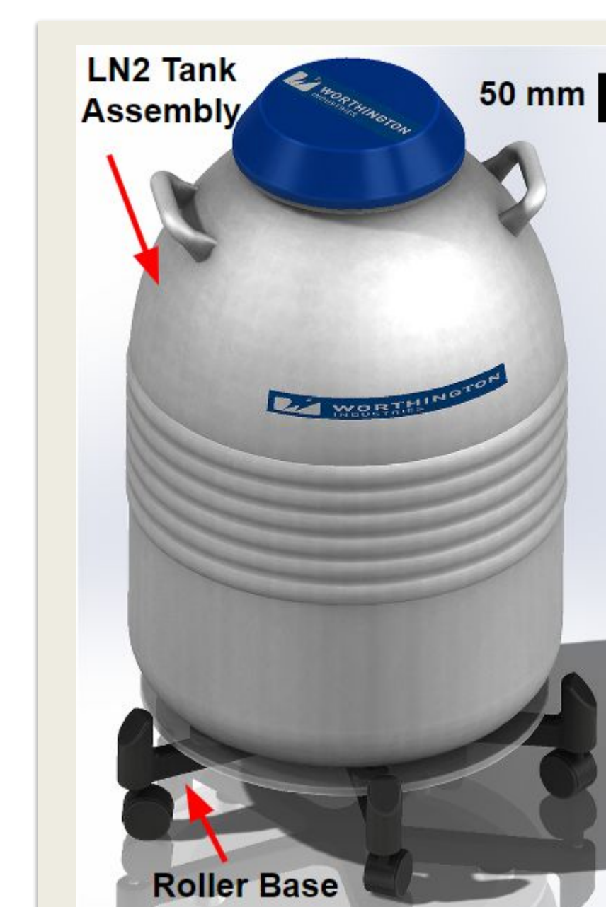
Figure 4: SolidWorks rendering of the fully assembled roller base and integrated scale with the LN2 tank placed directly on the assembly
