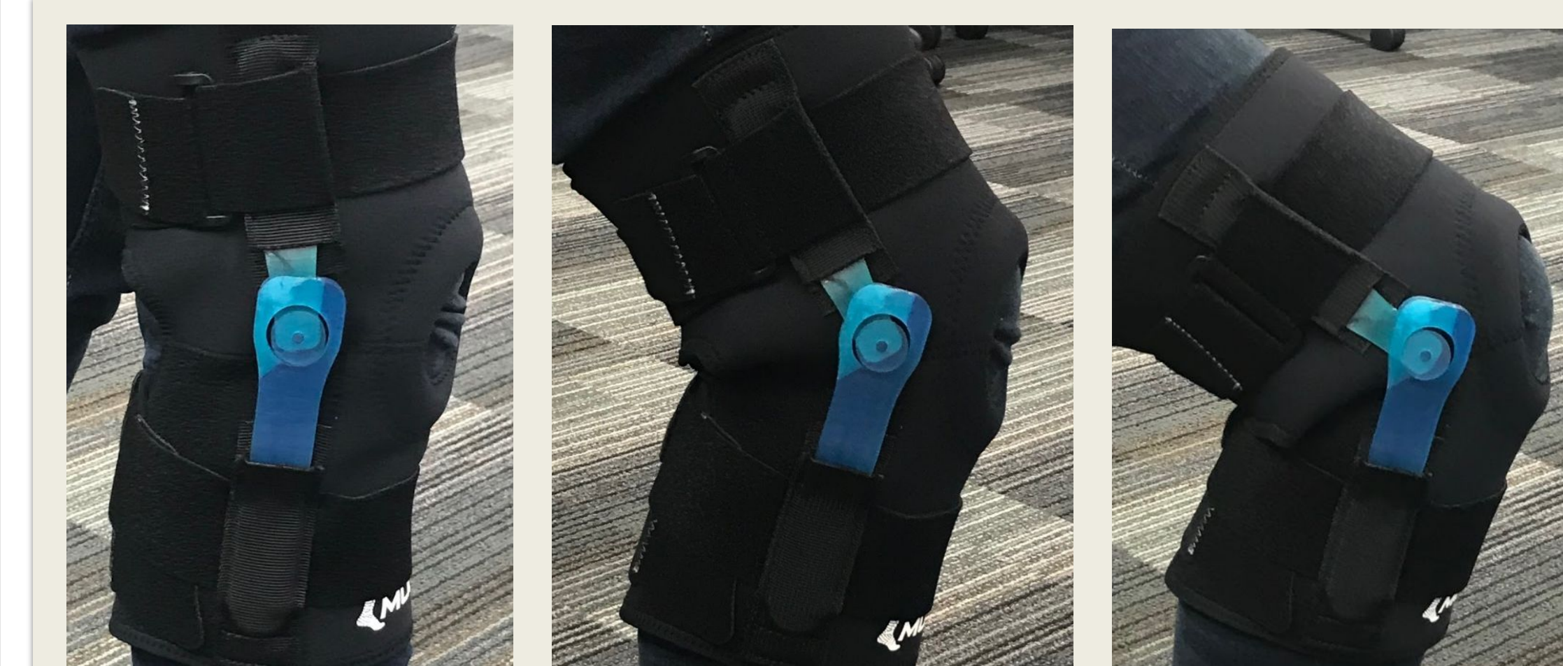
Figure 10: Step 5 - The hinge is in the sleeve, on the subject. The subject is performing activities leading to various degrees of knee flexion.
