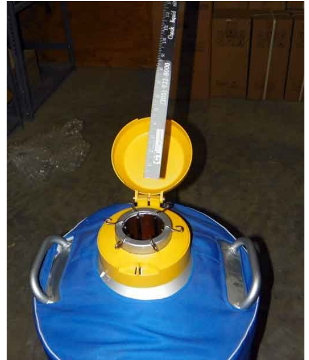
Figure 3: Simple measuring sticks are a quick and easy way to check LN2 levels.
