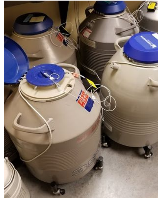
Figure 1: Small capacity LN2 storage tank used by our client Dr. Jeffrey Jones at the Generations Fertility Care clinic.
