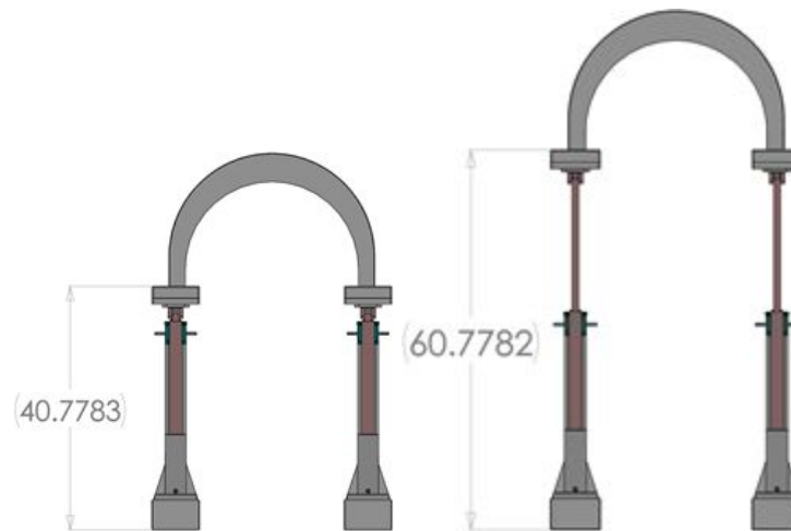
[Figure 21] The animation of the shield as is fully retracted (Left) to when it is fully extended above the patient (Right).
