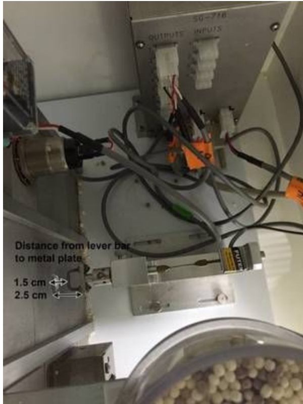
Figure 1: As shown in the picture above, the handlebar will be 2.5cm from the slot in the cage wall.
