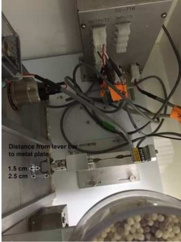
Figure 8: Picture of current system, handlebar will be 2.5 cm from the slot in the cage wall
