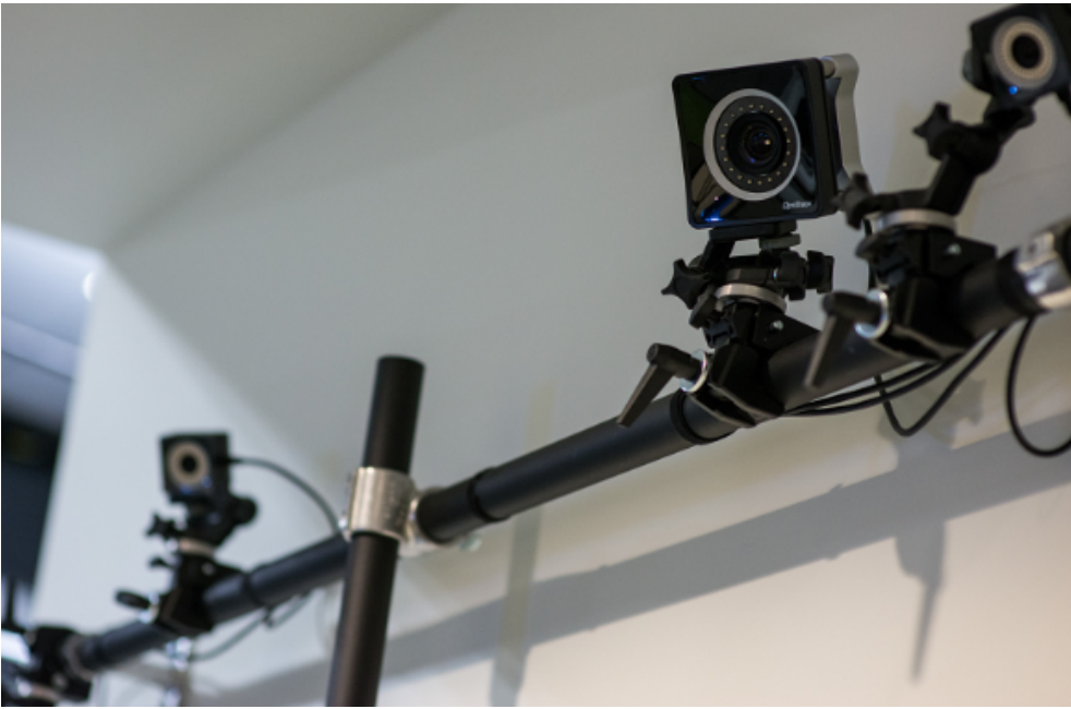
Figure 2: Tripod attachment which allows movement in 3 degrees
