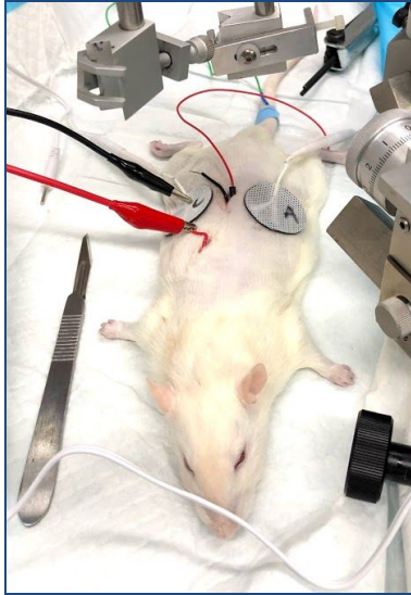
Figure 6. Post-Mortem Rat with Stimulation. A cathode and an anode were placed on either side of the spinal cord while two recording probes were used to measure the voltage generated at the lumbar portion of the spine.
