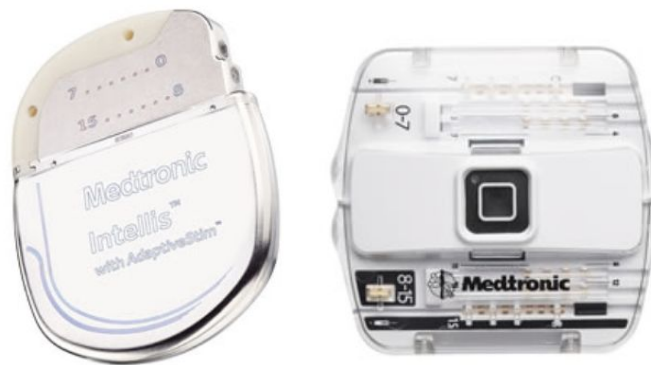
Figure 1: Medtronic Intellis Implantable Neurostimulator (left) [8] is a fully implantable neurostimulator that is used through wireless programming. This device is used in conjunction with the wireless external neurostimulator (right) which simplifies testing during trial and implant of the implantable stimulator.
