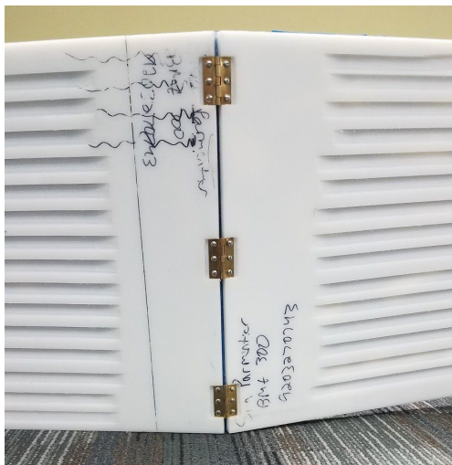
Image 14: A bottom view of the completed prototype, featuring the base plates and the dado cuts that were made into them to reduce their overall weight. Also shown are the affixed hinges and the milled pockets made to accommodate them.
