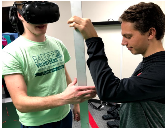
(Figure 2: A picture taken during testing showing a trial of the latency test in which a testee seeks to grab the yard stick as quickly as possible)
