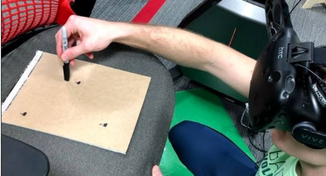
[Figure 9] A picture from the depth perception testing sequence in which a user seeks to accurately pinpoint an assigned location using a marker which represents a surgical tool.
