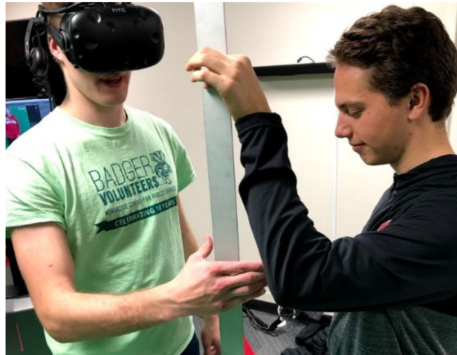
[Figure 11] A picture taken during testing showing a trial of the latency test in which a testee seeks to grab the yard stick as quickly as possible.
