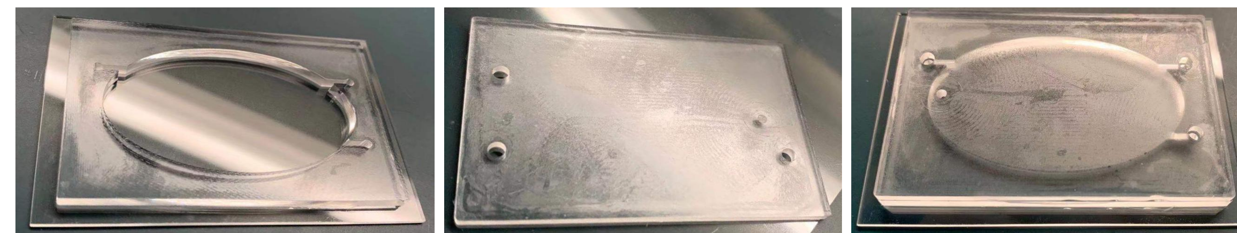
Figure 2.1: PDMS chamber layer and glass slide
