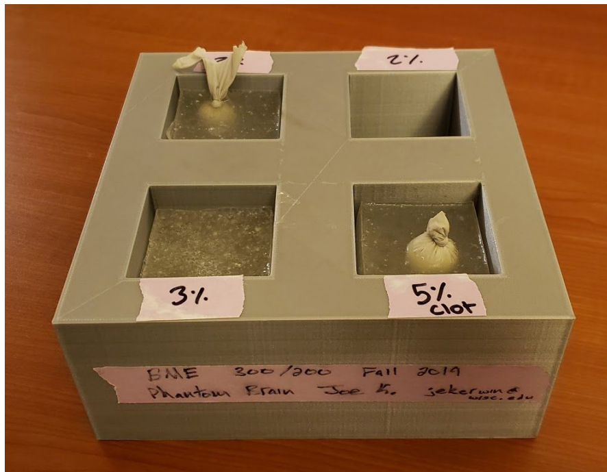
Figure 10: Sample holder containing three gel samples, two of which contain 2% base gels with 5% clots suspended, the third is a 3% gel alone.
