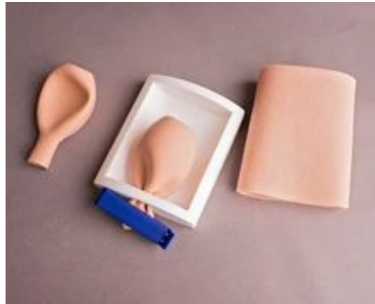
Figure 1: The cystocentesis trainer completed with a balloon tray
