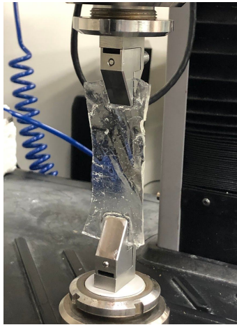
Figure 20: The tensile test set-up for the second specimen of the ecoflex gel - trial unit-- the Ecoflex 0030 setup mimics this
