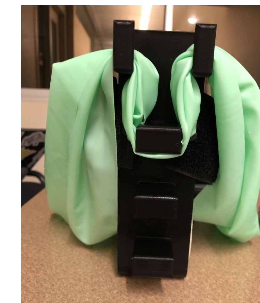
Figure 7: Back of the forearm trainer with a resistance band in place.
