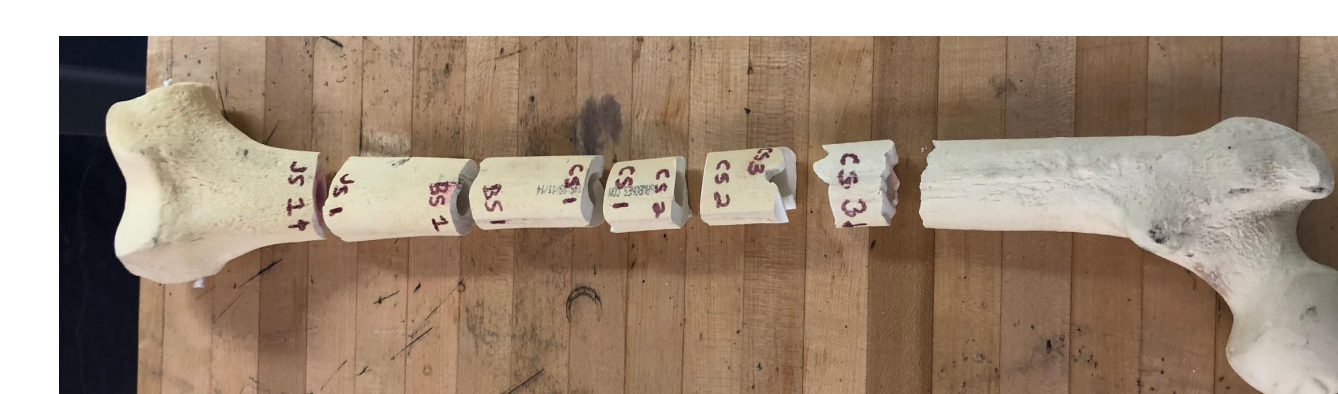
Figure 5: A bone model with practice cuts the team used for cut testing.
