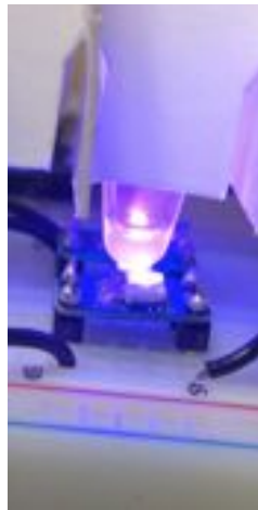
Figure 15: In vitro testing of KikGR cells with 405 nm LED. A lymph node cell suspension of KikGR cells was pelleted in a 1.7 mL clear, conical tube and placed directly on the 405 nm LED for 5 and 15 minutes with a 0 min exposure control (no exposure).
