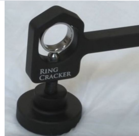
Figure 3&4. Ring cutter and ring cracker device
